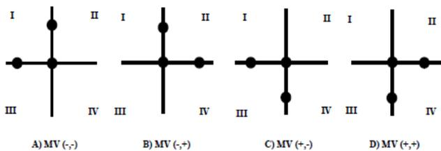
Fig.1 Direction of the current MV from the previous MV
