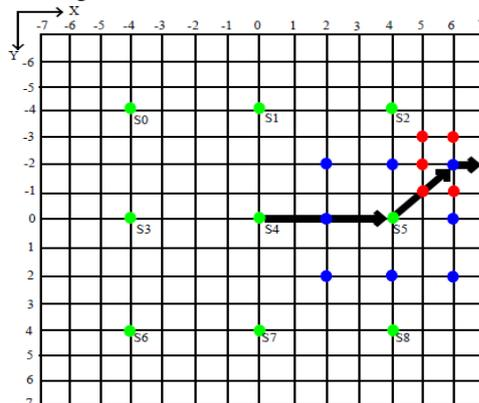
Fig.3 The FTSS Algorithm (the 9 search points in a step labelled by (S0- S8))
