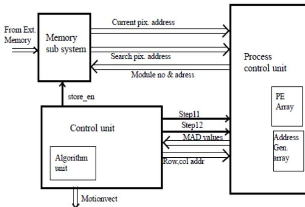
Fig.4 Block diagram of proposed architecture for FTSS Algorithm
