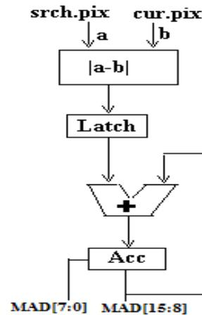
Fig. 5 Block diagram for processing element (PE)
