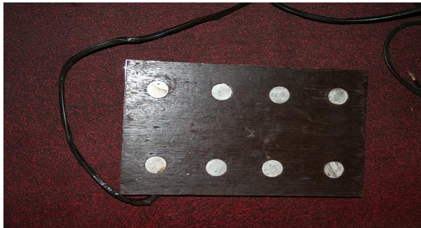
Fig.3: showing the front view of the active microstrip patch antenna
