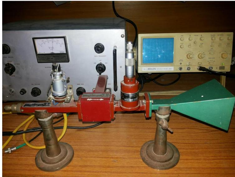
Fig. 4 Klystron microwave test bench
