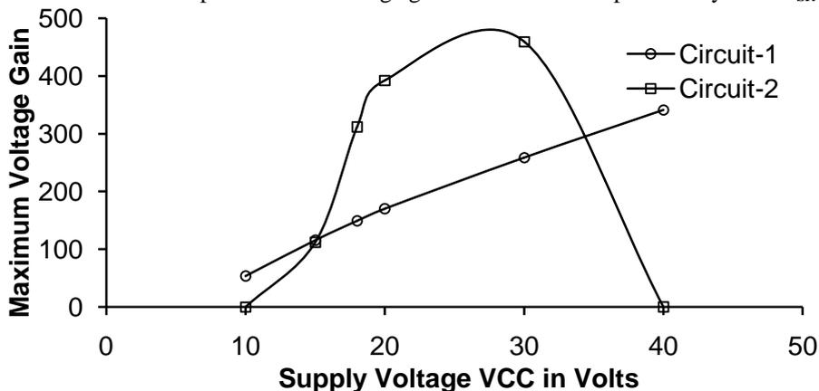
Fig.4. Variation of Maximum Voltage gain with Supply Voltage  $V_{CC}$
