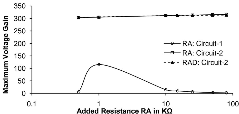
Fig.2. Variation of Maximum Voltage gain with Added Resistance RA and RAD
