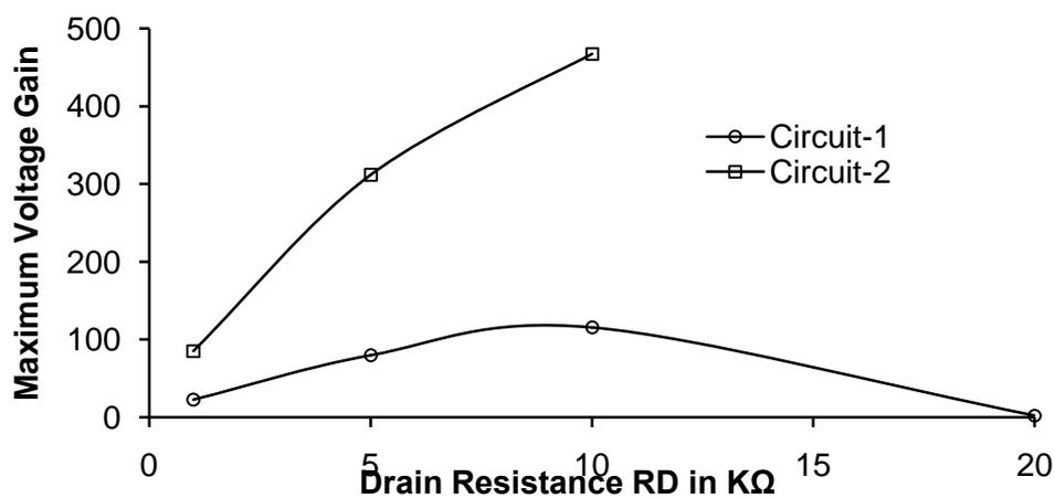
Fig.5. Variation of Maximum Voltage gain with Drain Resistance  $R_D$  or  $R_{CD}$
