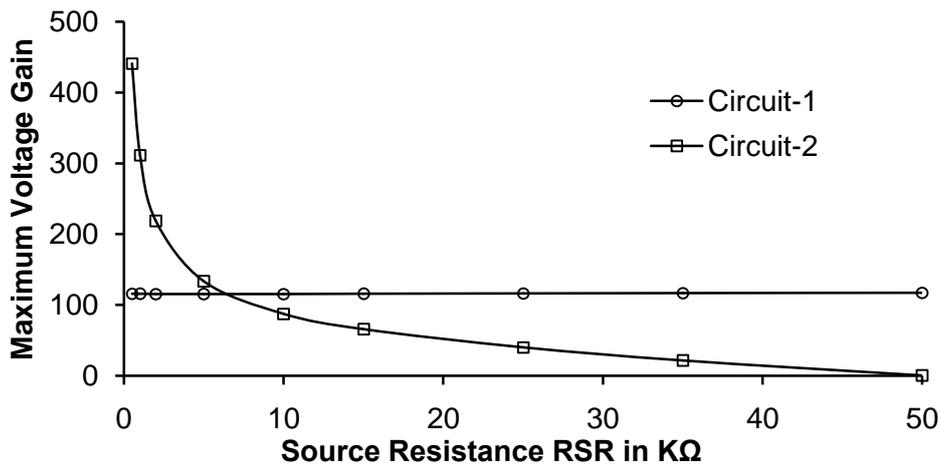
Fig.3. Variation of Maximum Voltage gain with Source Resistance  $R_{SR}$
