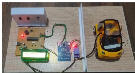
Fig 2: System prototype of RFID based EV charging station.
