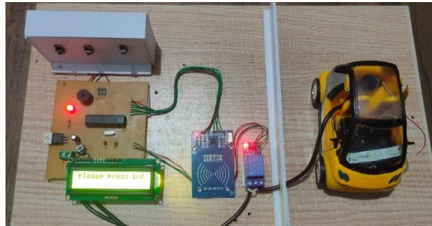
Fig 5: System prototype of RFID based EV charging station.
