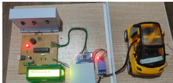
Fig 3: System prototype of RFID based EV charging station.
