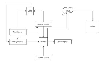
The LCD display can be used to display the power consumption data locally. The transformer is used to step down the voltage from the mains supply to a safe level for the ESP32 microcontroller.
