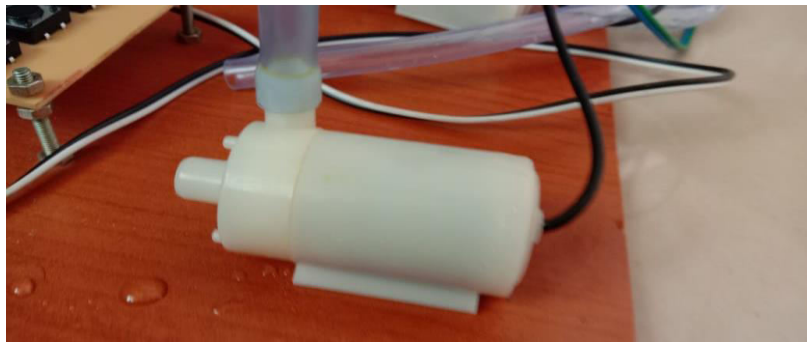
Figure 5. Dc motor with pump
