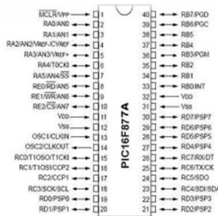
Fig-5: Pin Diagram Of PIC16F877A
