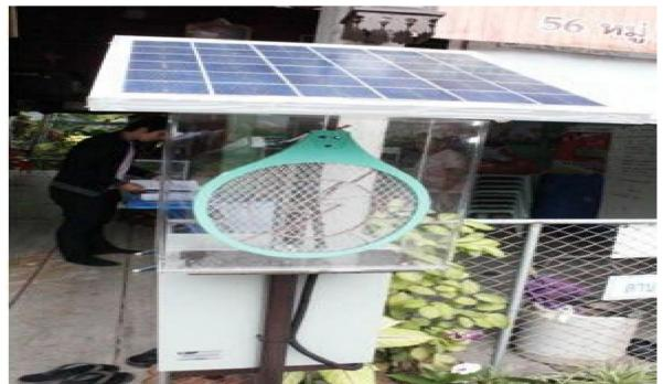
Fig 3.2.1 Solar Energy-Based Insect Pest Trap
