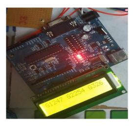
Fig 3(b) LCD Shows the Gas concentration
