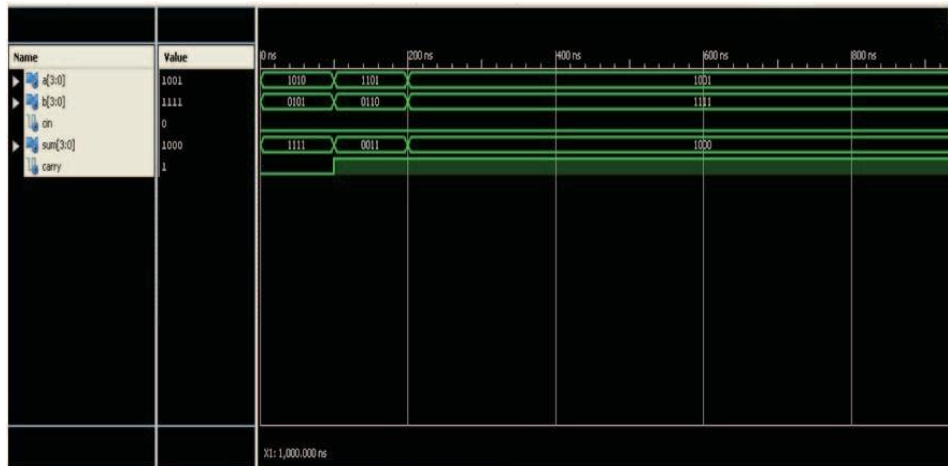
Fig. 10. Simulated waveforms 4-bit Modified Carry Select Adder.
