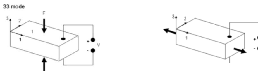
Fig. 3 Poling direction. 33 mode and 31 mode respectively
