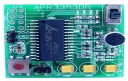
Figure 4. Voice recording/Playback unit
