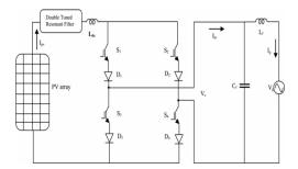
Fig. 1 Single phase grid connected CSI.
