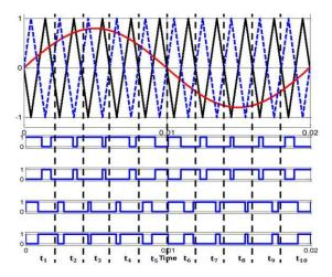
Modified carrier based PWM is proposed to control the switching pattern for the single phase grid connected CSI. To provide a continuous path for the dc side current, at least one top switch in either arm and one bottom switch must be turned on during every switching period. In this fig. 4 shows reference and carrier waveform along with switching patterns. The carrier with solid line. The straight for upper switches while dashed line is lower switches
