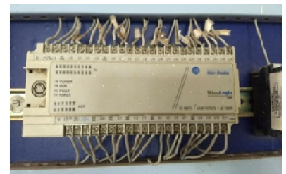
Figure3: Micrologix 1000 total input signals : 20 total output signals : 10 input voltage: 24v output voltage: 24v power supply :24v / AC 230
