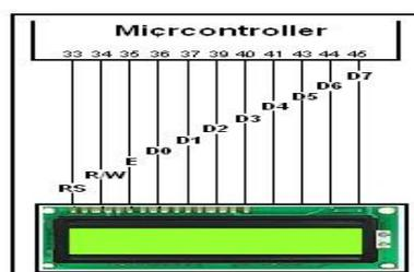
Fig 7: Microcontroller and LCD Interface
