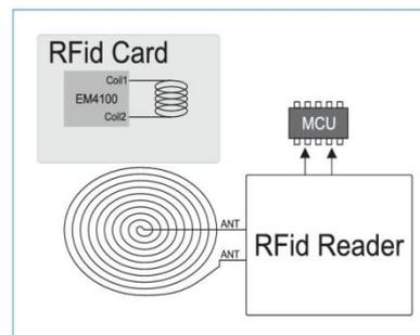
Fig 11: Principle of RFID reader operation
