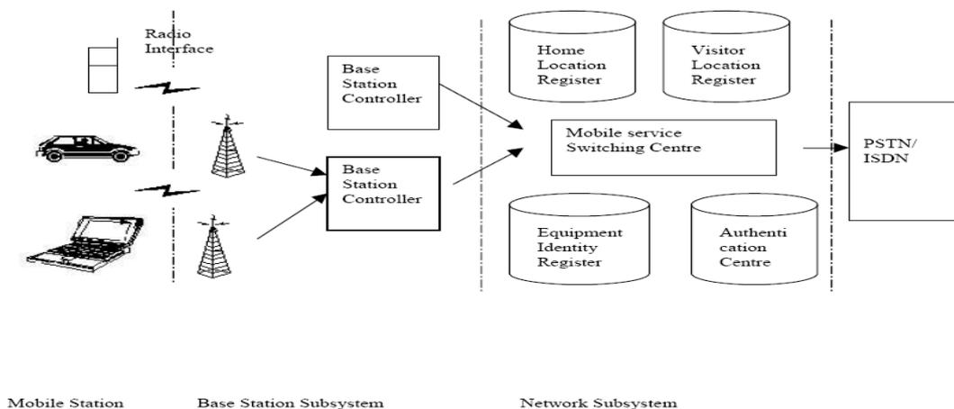
Fig 6: Architecture of GSM
