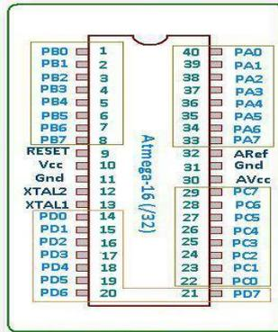
Fig 3: Pin configuration of AVR (Atmega16)
