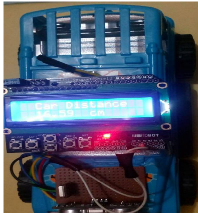
Fig 2 Ultrasonic sensor,RF transmitter and LCD Display mounted on a toy car (vehicle one)
