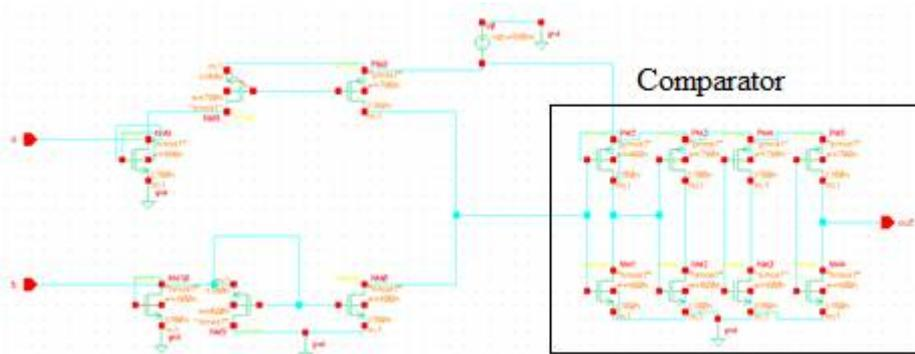
Figure 11. Current mode comparator
