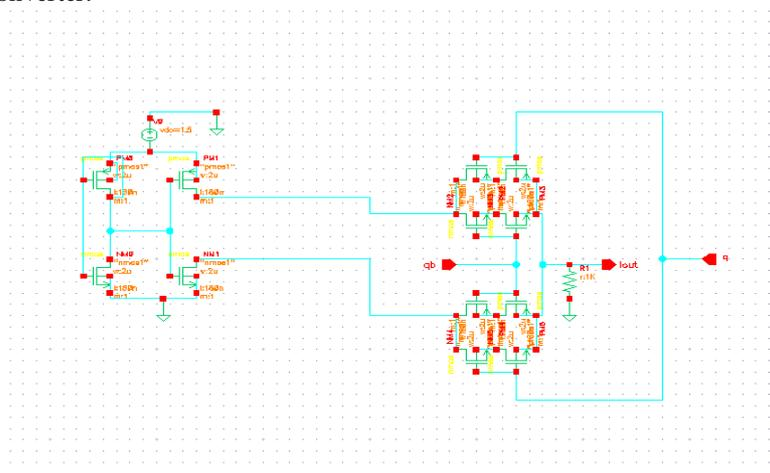
Figure 7. Current mode Digital to Analog converter
