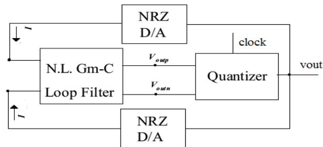
Fig. 1 Proposed modulator block diagram in [1]
