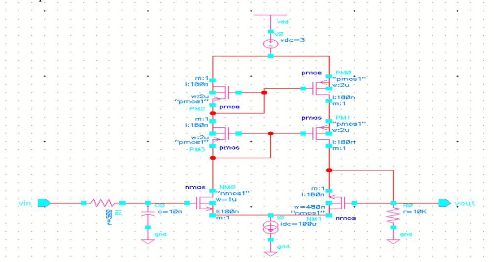
Figure 3. CMOS OTA based filter.
