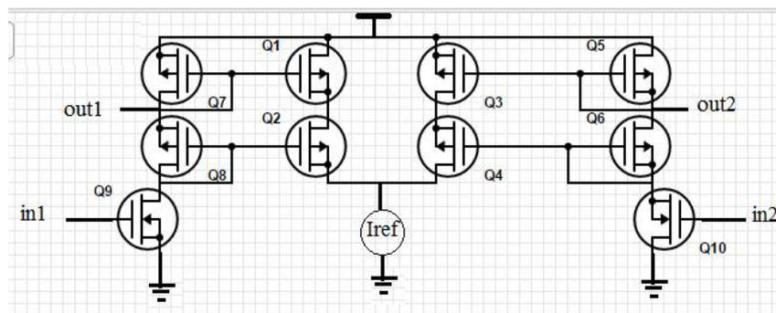
Figure 5. Current mirror based Digital to Analog converter[9].
