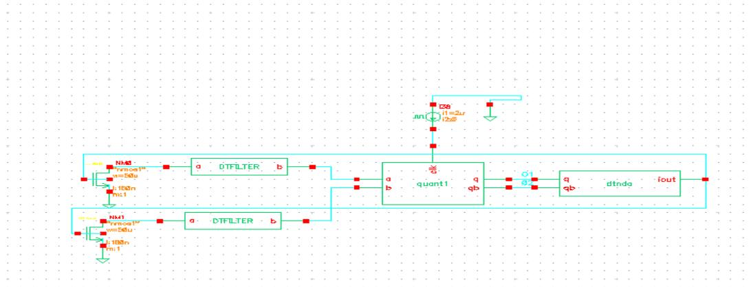
Figure 10. DT MOS based sigma delta modulator
