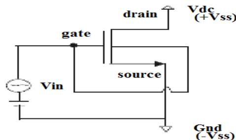
Fig. 2 DTMOS transistor
