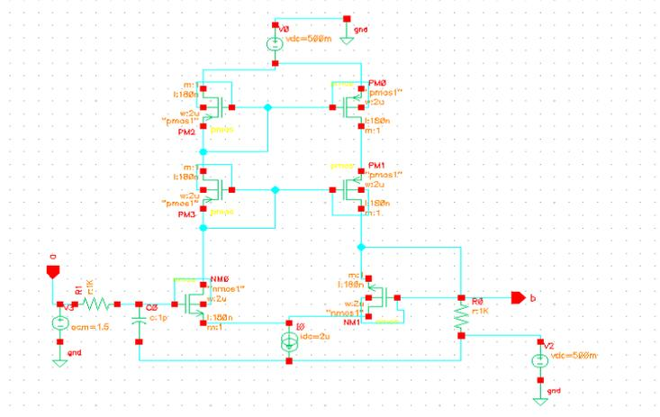
Figure 4. DTMOS based OTA filter
