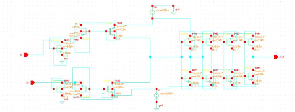
Figure 12. DT MOS based Current mode comparator.
