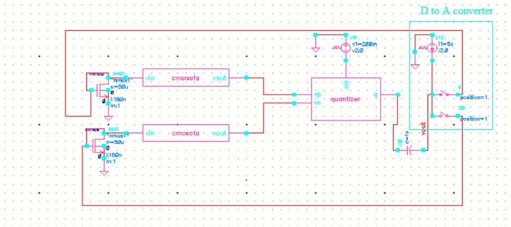
Figure 9. OTA based Modulator with Digital to Analog converter.
