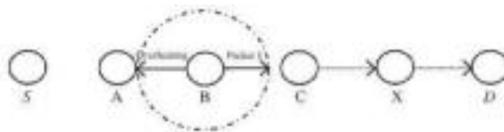
Above figure shown the example of limited power transmission in order to preserve its self battery resources, node B intentionally check its transmission power so that it is strong suitable to be overhead by node A but not strong suitable to be received by node C.
