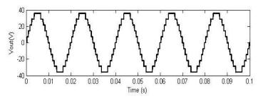
Fig 6. Simulated Output Voltage Of Eleven Level Symmetric Inverter
