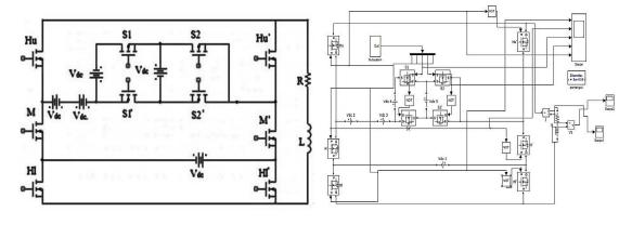
Fig 4. Circuit diagram of eleven level inverter
