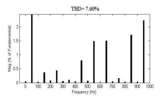
Fig 8. Total Harmonic Distortion Of Eleven level Symmetric Inverter
