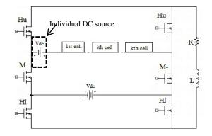
Fig 1. Overall view of symmetric multilevel voltage source inverter.
