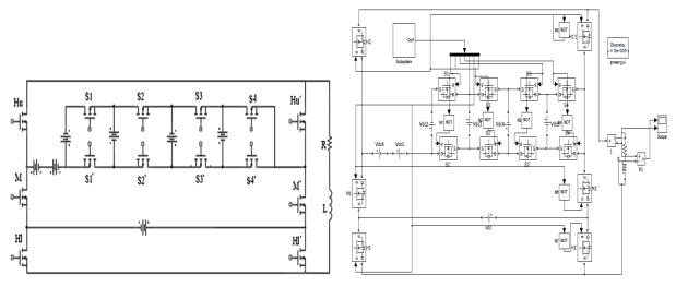
Fig 8. Circuit Diagram Of The Fifteen Level Inverter
