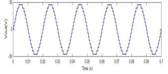
Fig 10. Simulated Output Voltage Of Fifteen Level Symmetric Inverter
