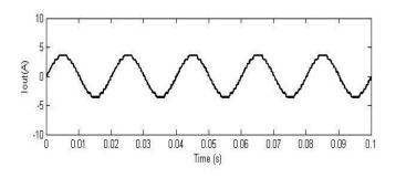
Fig 7. Simulated output current Of Eleven Level Symmetric Inverter
