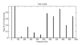
Fig 12.Total Harmonic Distortion of Symmetric Fifteen-Level Inverter
