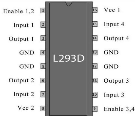
Fig 4 Pin diagram of L293D.
