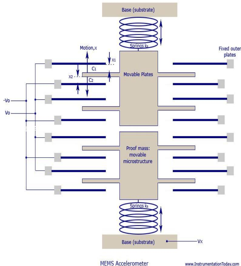
Fig 1. MEMS accelerometer sensor
