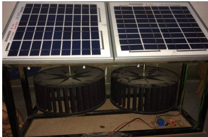
Fig.1 Model of Proposed hybrid solar-wind system
