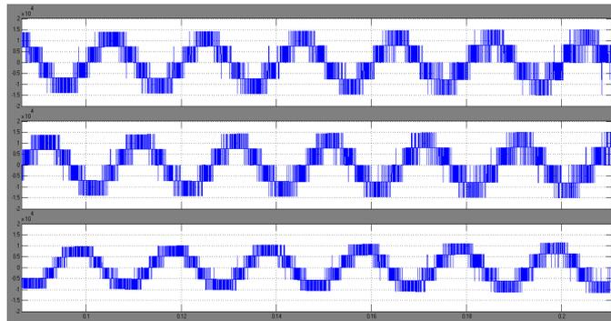
Fig.15 Five Level Output Voltage
