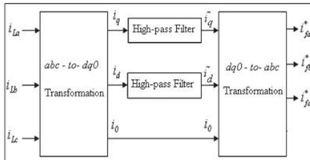
Fig.4 Proposed controller based on the d-q-0 theory
