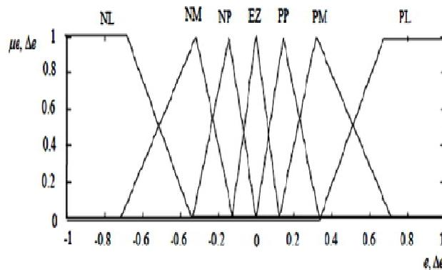
Fig.8 Membership functions for Input, Change in input, Output.
