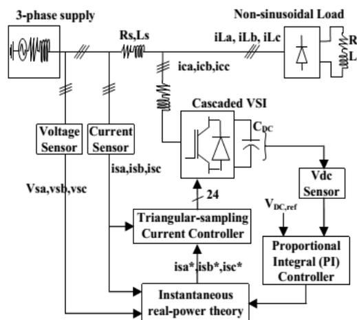
Fig 1 Shunt Active Power Line Conditioners System
