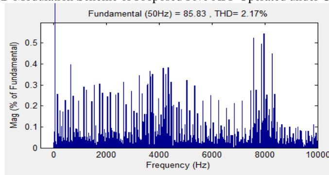
Fig.18 FFT Analysis of Source Current
