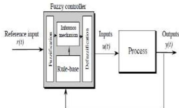
Fig.6. General Structure of the fuzzy logic controller on closed-loop system
