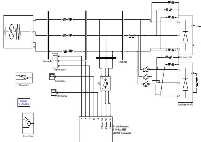
Fig.9 Matlab/Simulink Mode of Proposed Five APF Operated under Classical PI Controller
