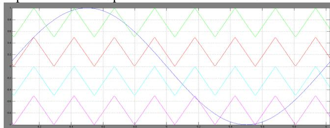
Fig. 17 Switching States- IPD Modulation Scheme
