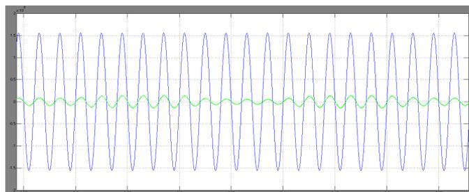
Fig.13 Source Side Voltage & Current in In-Phase Condition
