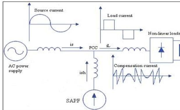
Fig.5 Main power circuit (SAPF in a four-wire distribution network)
