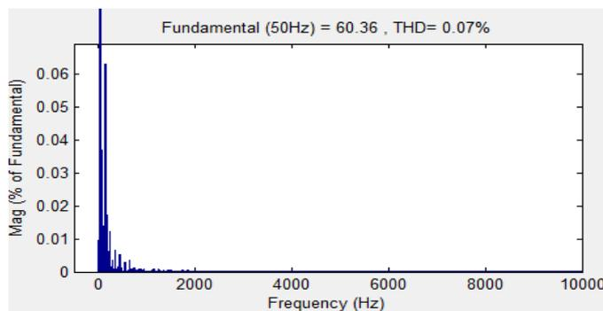
Fig.21 FFT Analysis of Source Current
