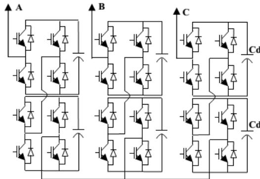
Fig 2 Design of cascaded multilevel active power filter
