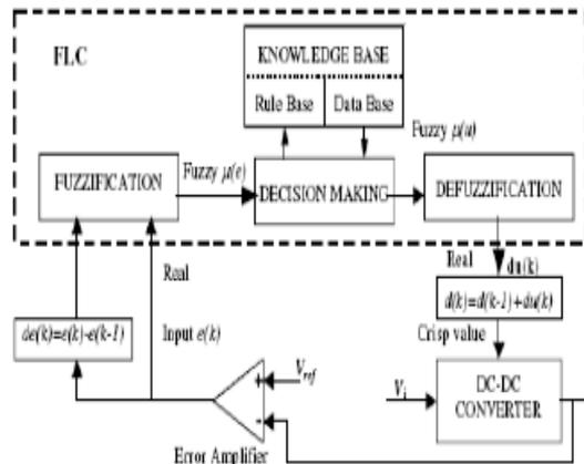
Fig.7. Block diagram of the Fuzzy Logic Controller (FLC) for dc-dc converters
