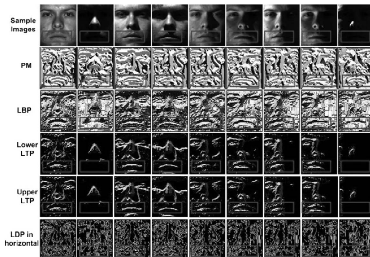
Fig. 3 Analysis of various pattern based methods on sample face images under illumination changes. PM: proposed method (LDMaMEP)
