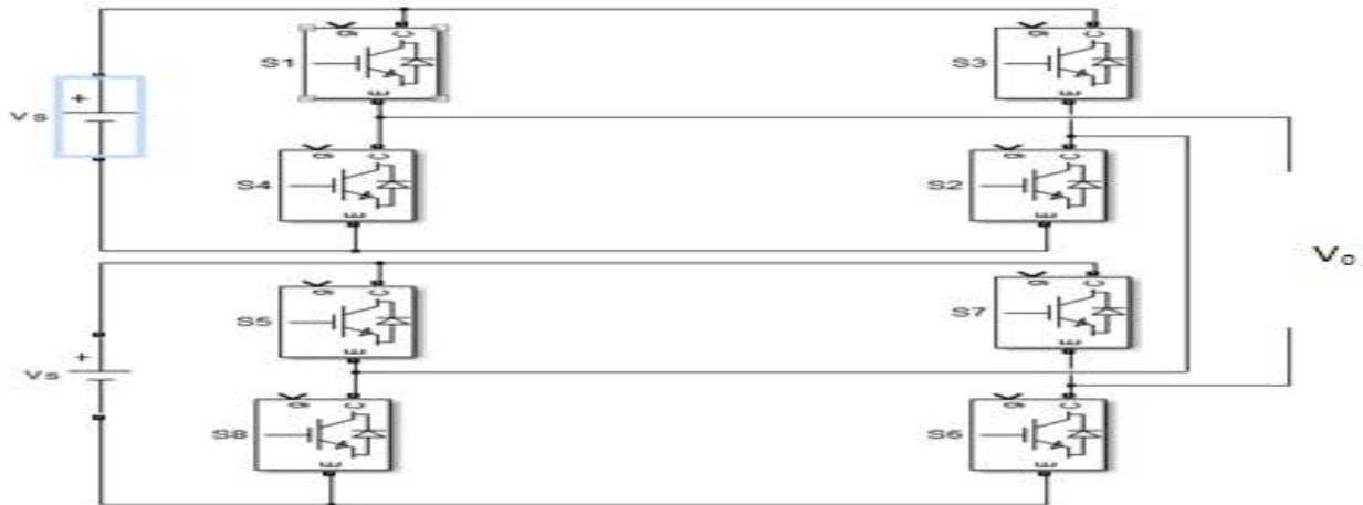
Fig. 3: Single phase five level cascaded VSI
