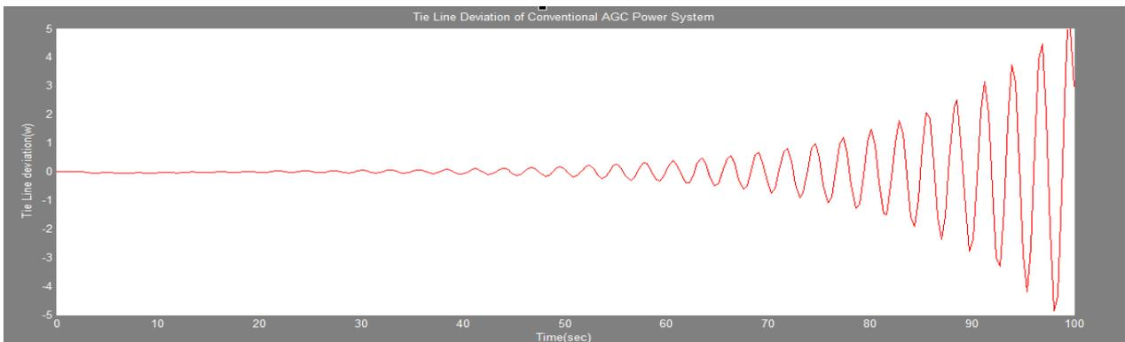
**Fig 8(c)Tie line deviation of conventional PID two areas AGC system**
