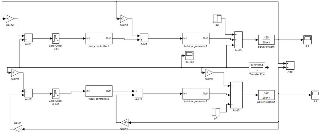
Fig3 Block diagram of two area power system for LFC
