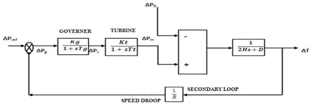
**Fig1: Block diagram representation of AGC system**
