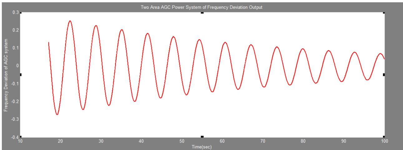
Fig8(a) Frequency deviational of Conventional PID AGC system
