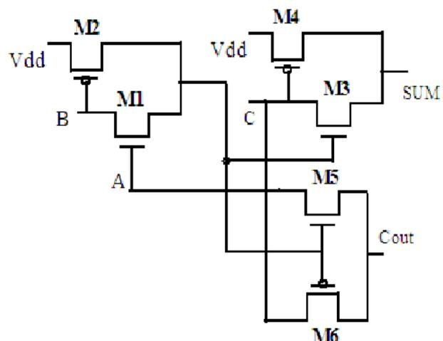
Fig .5: Full Adder using 6T.
