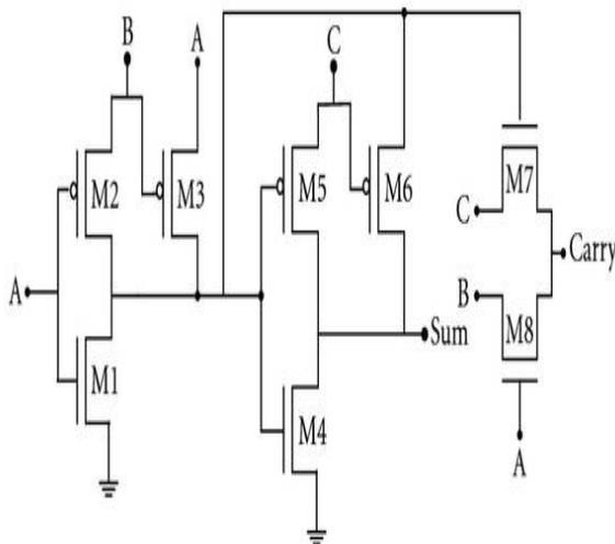
Fig.4: Full Adder using 8T
