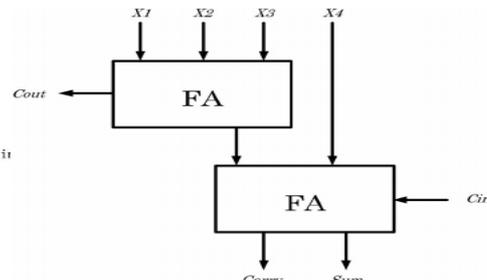
Fig.8: 4:2 Compressor using Two Full Adder.
