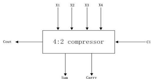
Fig.7: Block diagram of 4:2 compressor circuit.
