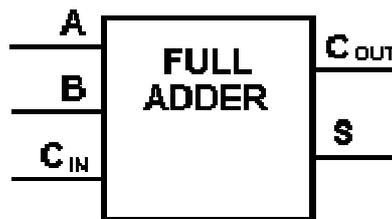
Fig.1: Block diagram of 1-bit Full Adder circuit.
