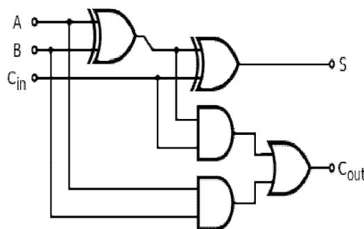
Fig.2: Static Design of Full Adder circuit using Gates.
