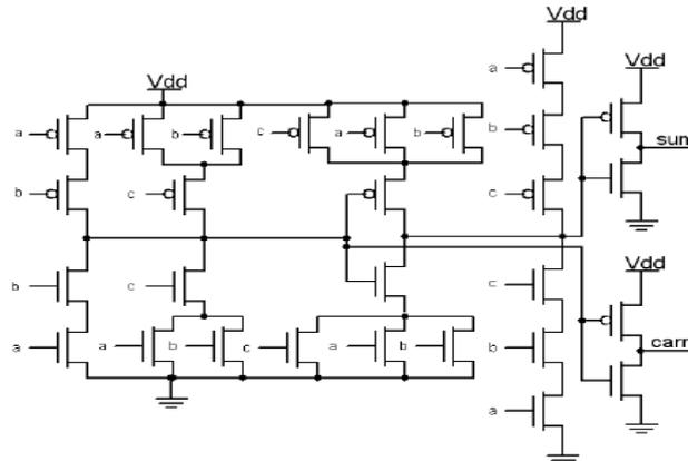
Fig.3: Full Adder using Static design 28T.
