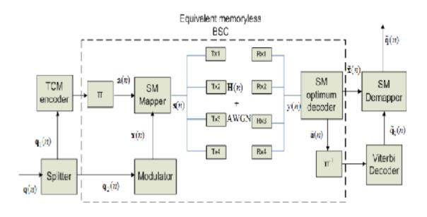
Figure 1: Block diagram for proposed TCSM system
