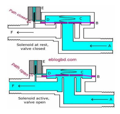
Solenoid valve are also characterized by how they operate. A small solenoid can generate a limited force. If that force is sufficient to open and close the valve then a direct acting solenoid valve is possible.
