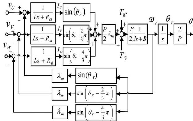
Fig. 7. PM synchronous motor block diagram.
