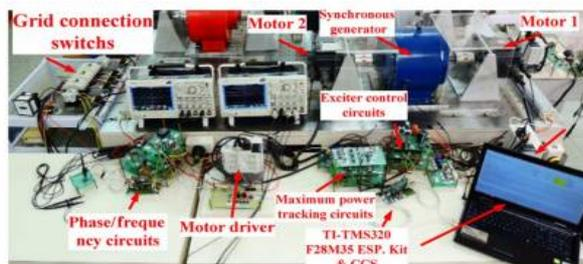
Fig. 11. Photograph of experimental setup
