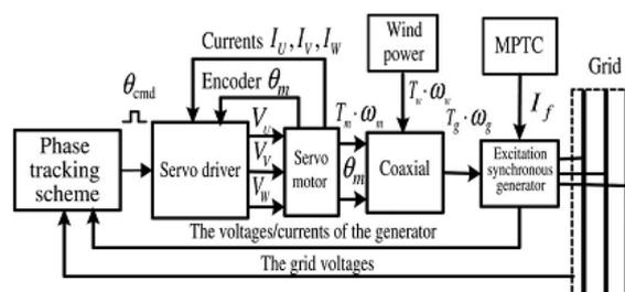
Fig. 5. Proposed wind power generator system
