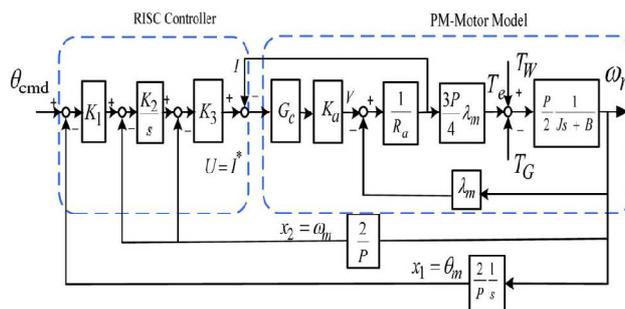
Fig. 8. Servo motor position control loops.
