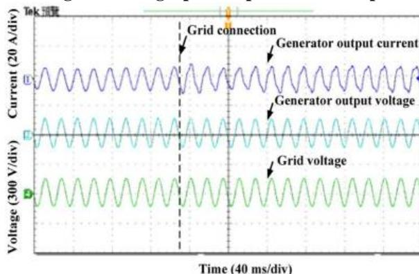
Fig. 12. Generator output current and voltage versus grid phase voltage
