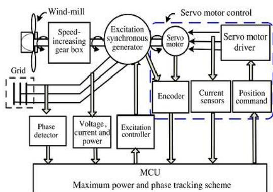
Fig. 4. Proposed wind power system framework.
