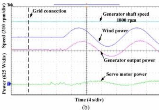
Fig. 13. Maximum power tracking experimental results. (a) Wind power step changes. (b) Wind power sine wave changes.
