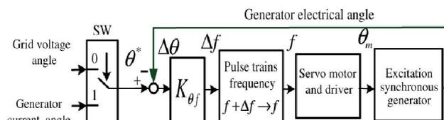
Fig. 9. Phase tracking control scheme.
