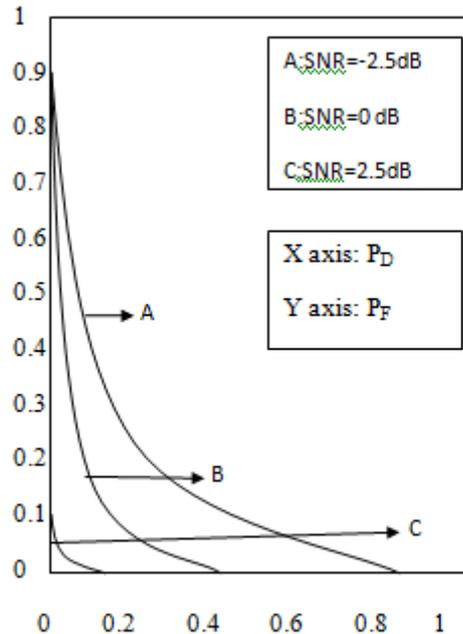
SNR also affect the performance of the energy detection technique. Figure shows the energy based spectrum sensing under different signal to noise ratio.
