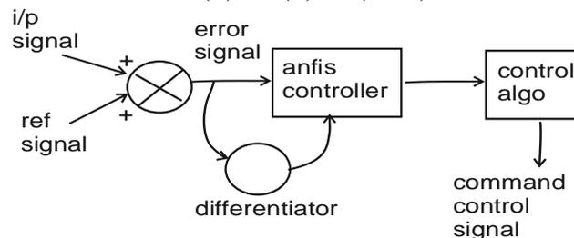
Fig. 2 : Illustration of a typical ANFIS Controller with 2 Inputs
