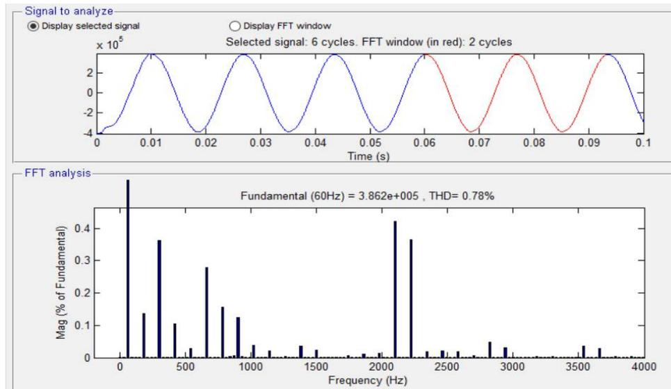
Fig. 11 : Waveform showing the THD after applying compensation using ANFIS (i)
