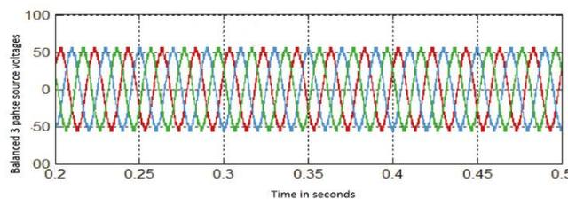
Fig. 6 : Matlab output of balanced 3-phase source voltages after incorporation of ANFIS (Artificial Neural Network's Neuro-Fuzzy) controller
