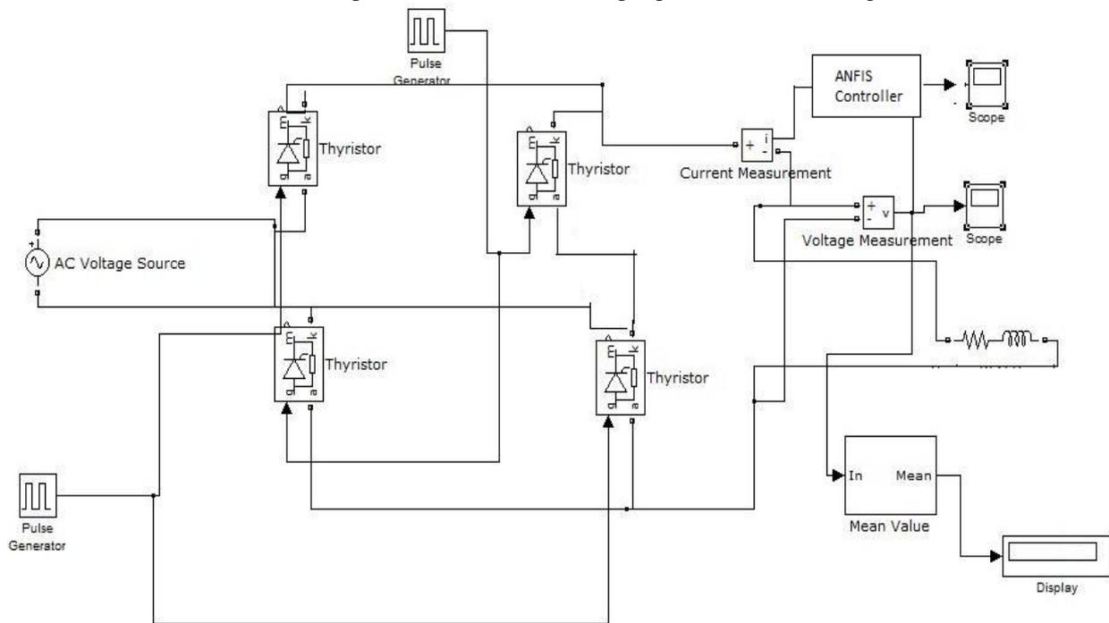
Fig. 4 : Developed simulink model for ANFIS controller for harmonic eliminations
