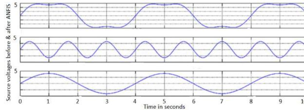
Fig. 5 : Simulation output for the plot of load voltage before and after the incorporation of the ANFIS (artificial neural network's neuro-fuzzy) controller .... before, imbalance seen due to switching, after the incorporation of the ANFIS controller, balance is seen
