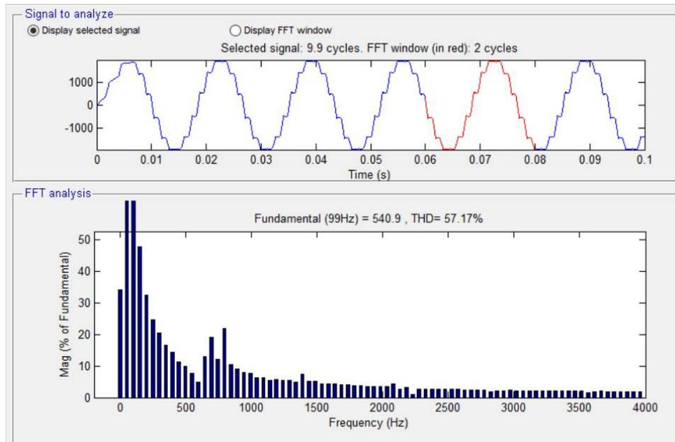
Fig. 10 : Waveform Showing the THD Before Applying Compensation Using ANFIS (I)
