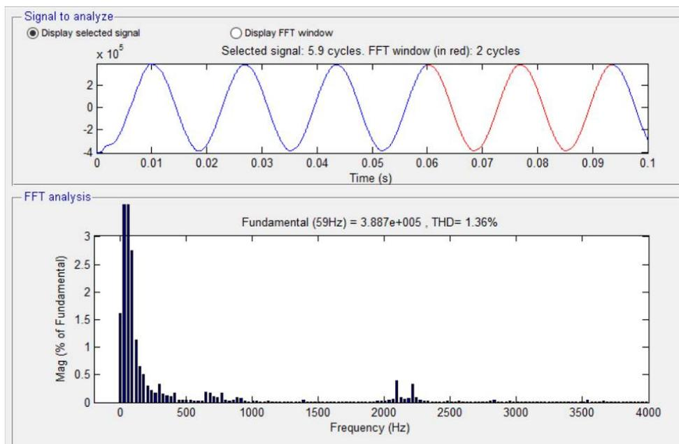
Fig. 9 : Waveform Showing the THD after Applying Compensation Using ANFIS (V)
