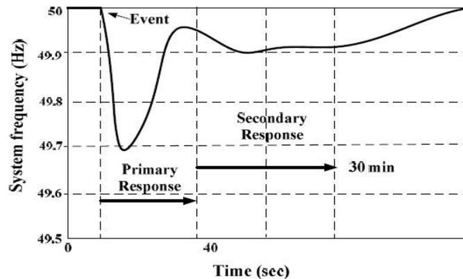
Fig 5. Definitions of frequency control in power systems
