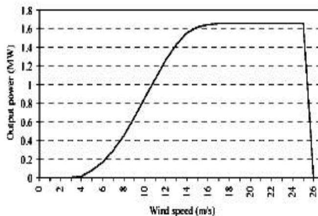
Fig-1 Power Curve for VESTAS V66-1.65 MW Wind Turbine
