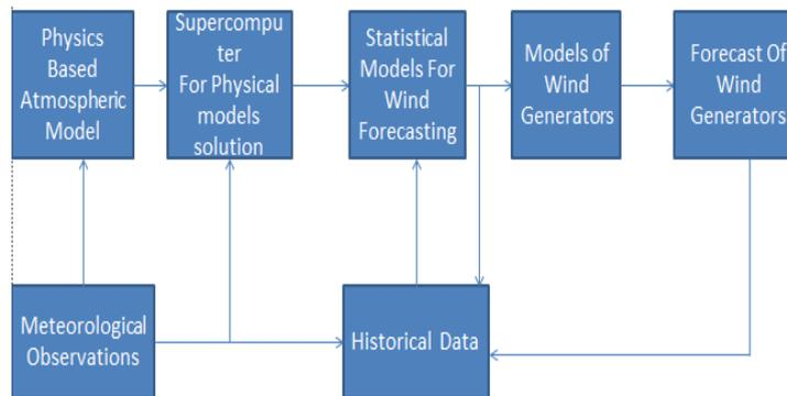
Fig 3. Hybrid Approach of Wind Power Forecasting
