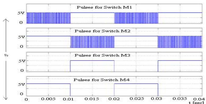
Fig3. Switching pattern for the MOSFET switches of converter
