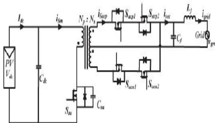
Fig 8: Flyback inverter scheme
