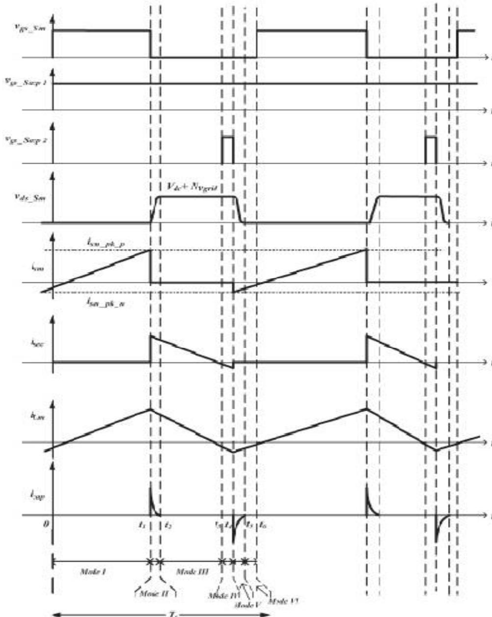
Fig 9: Detailed operation of inverter scheme
