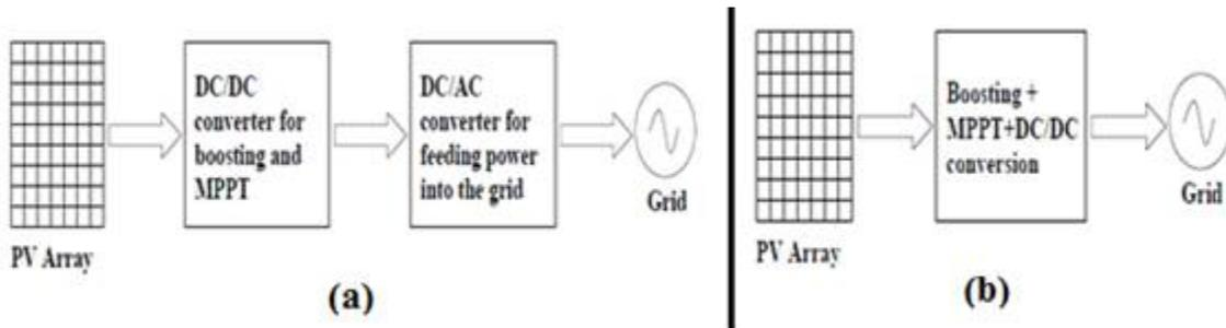
Fig 1: (a): Multi stage configuration (b): Single stage configuration
