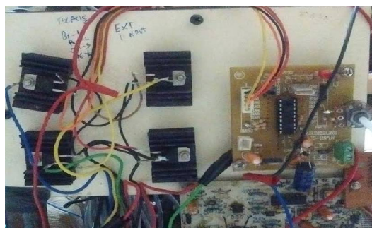
Fig 7: The microcontroller-stepper motor driver circuit
