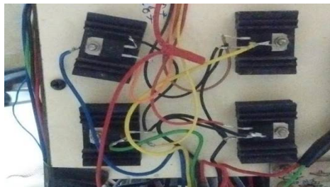
Fig 6: The stepper motor driver circuit.
