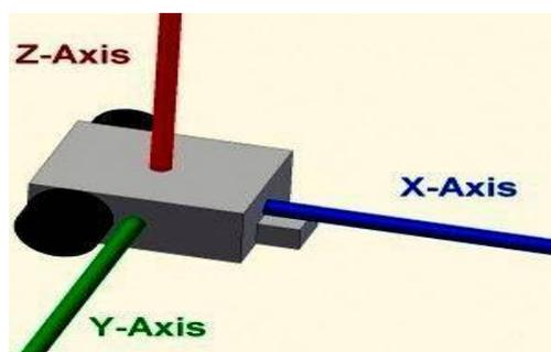
Fig. 1 sensing direction of the tri-axial MEMS accelerometer.
