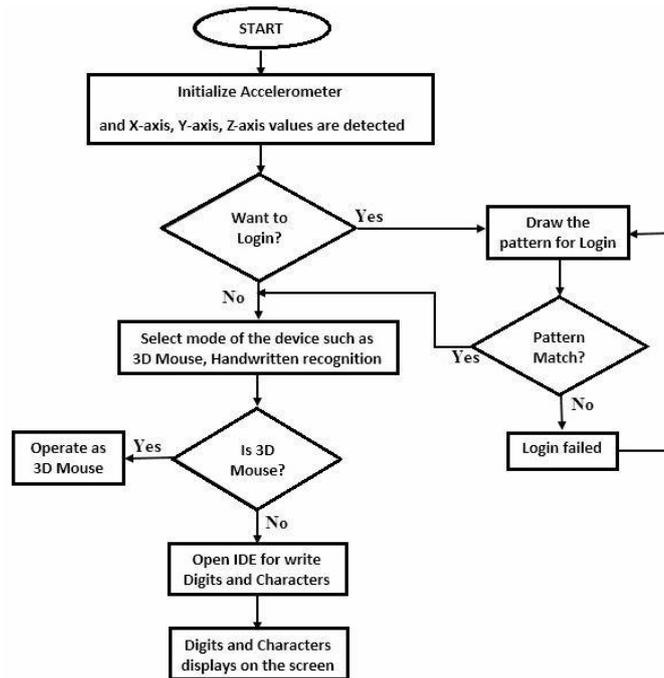
Fig. 4 Flowchart of MEMS accelerometer based system process
