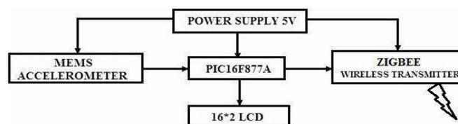
Fig. 2 Block diagram of transmitting module.
