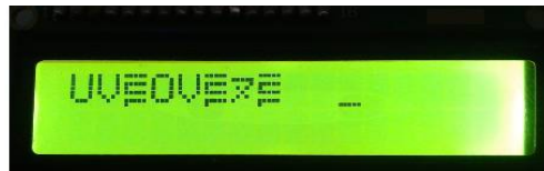
FIG 5.1. LCD DISPLAY OF UNDER VOLTAGE
