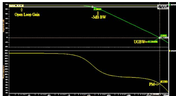
Fig. 8. AC analysis of Op-amp
