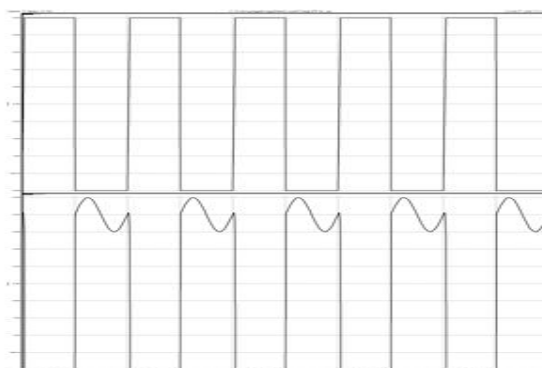
Figure 6. Waveform of PFAL based Inverter
