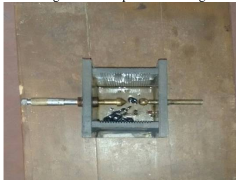
Fig. 2 Arrangement of electrodes and insulating paper for Sphere-Cone electrode configuration.
