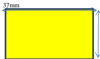
Fig. 1. Conventional Rectangular Microstrip Patch Antenna
