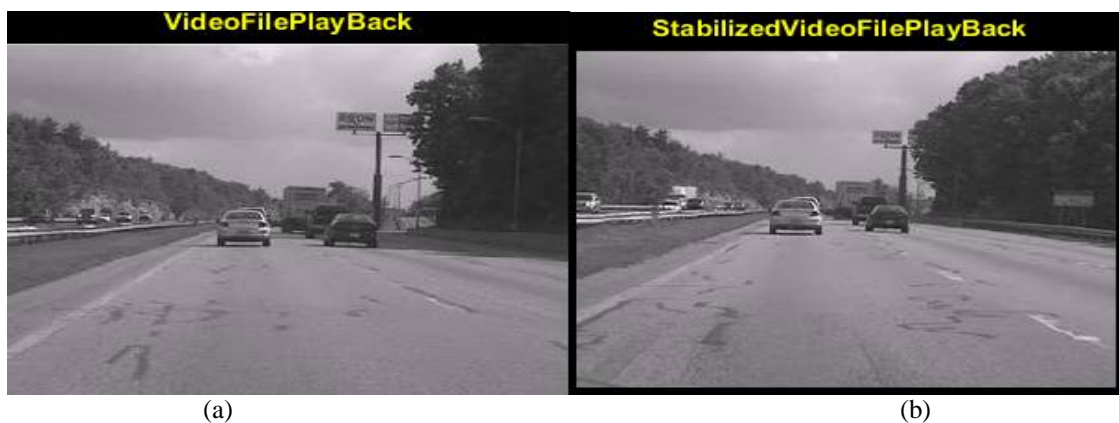
Fig 4:(a) Unstable input frame (b)Stable output frame for “Shaky Car” video frame.
