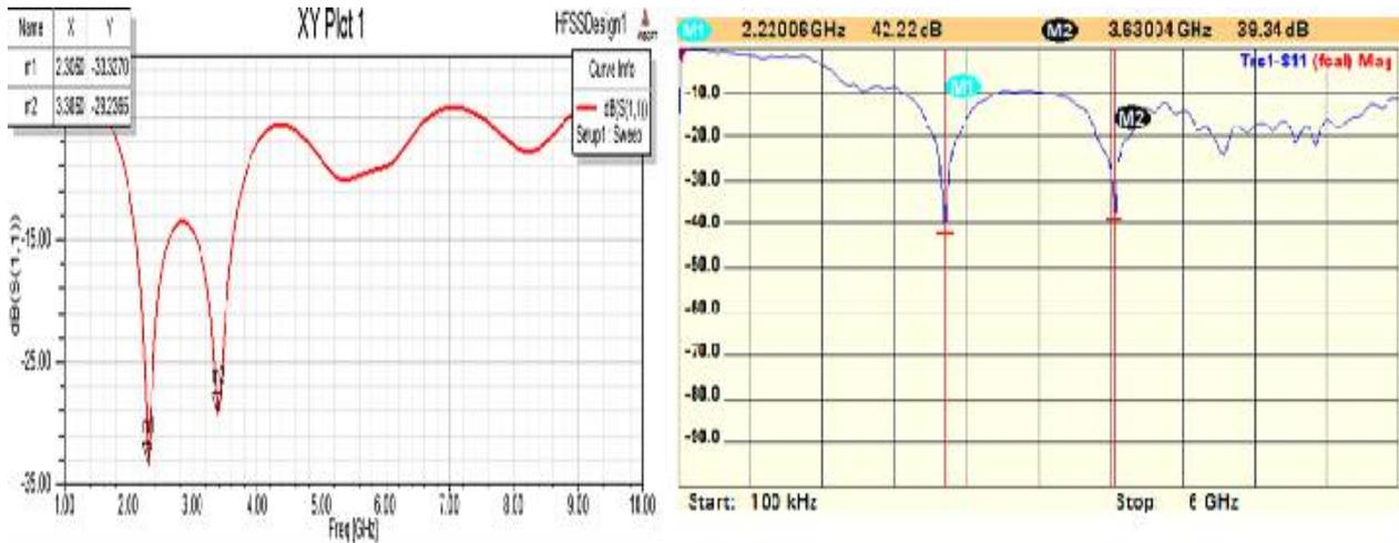
Fig. 4 Simulated and measured Return loss of the proposed wideband antenna.
