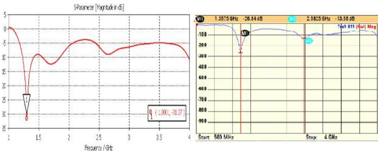
Fig. 5 Simulated and measured Return loss of the proposed narrowband antenna.
