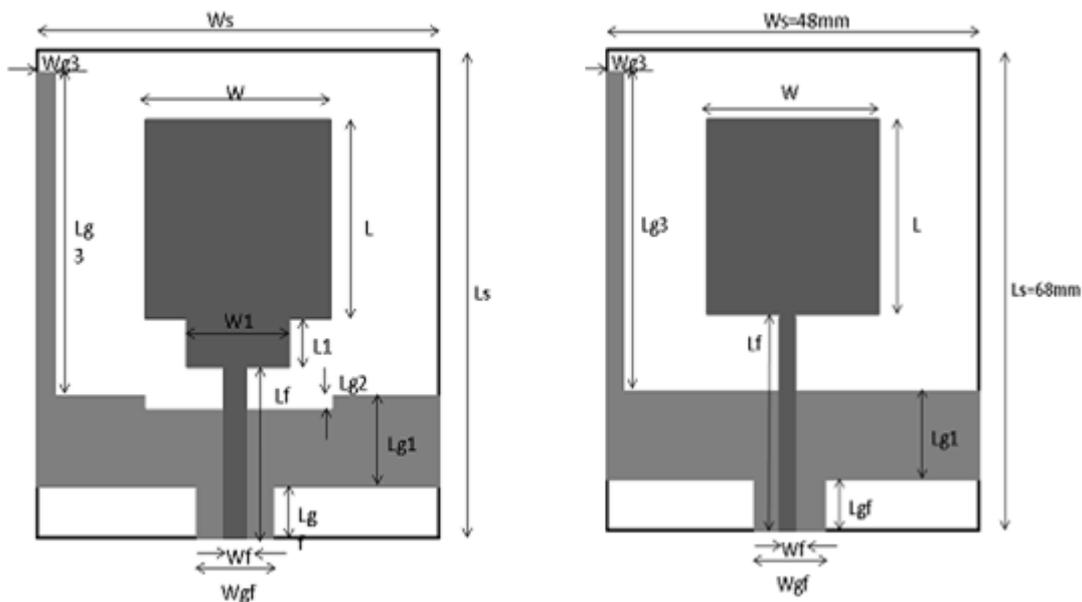
Fig. 3 Configuration of the proposed wideband and narrowband antenna.
