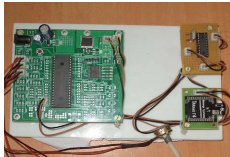
Figure 9. The Engine Control Module which includes 3 ADC sensors, WCAN and Tarang RF Module
