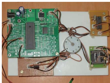
Figure 11. The D.C. Motor Module includes the DC Motor and the Temperature Sensor
