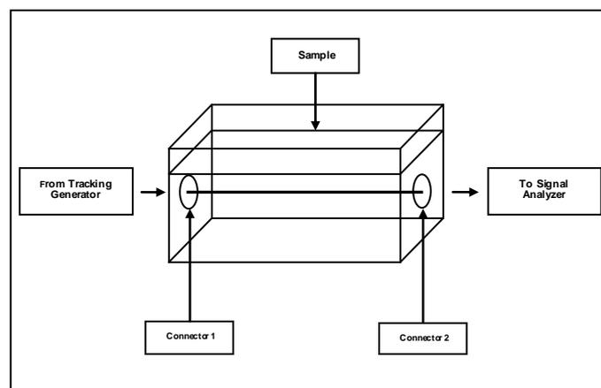
Fig. 1: Schematic of the Measurement Cell
