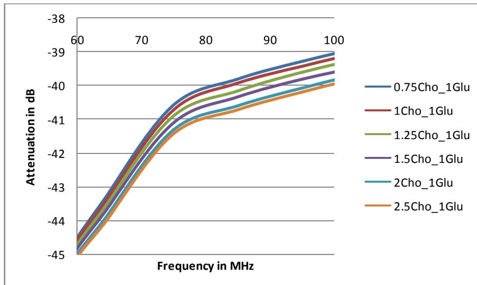
Fig. 3: Graph of 60MHz - 100MHz with normal Glucose concentration
