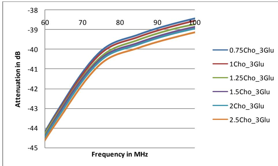
Fig. 6: Graph of 60MHz – 100MHz with 3 times the normal Glucose concentration
