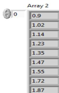
The above front panel indicates the corresponding for each and every cm of level. For '0 cm' of level, the corresponding voltage from transmitter is 0.9 V and for '1 cm' of level, the corresponding voltage from the transmitter is 1.02 V. similarly for every cm of level, the corresponding voltage is displayed.
