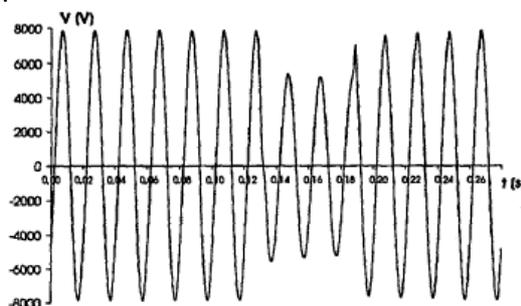
Fig. 1 Typical waveform of voltage sag
