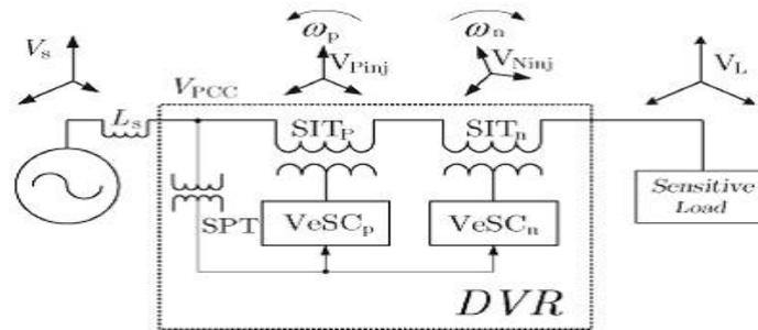
Fig. 7 Block diagram of two- module VeSc based DVR
