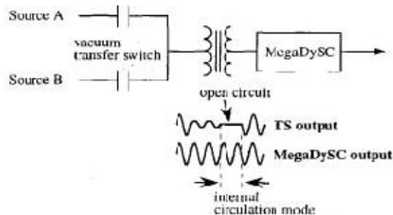
Fig. 4 Ultra-reliable power is supplied cost-effectively by using a vacuum transfer switch plus a voltage sag corrector with ride-through capability
