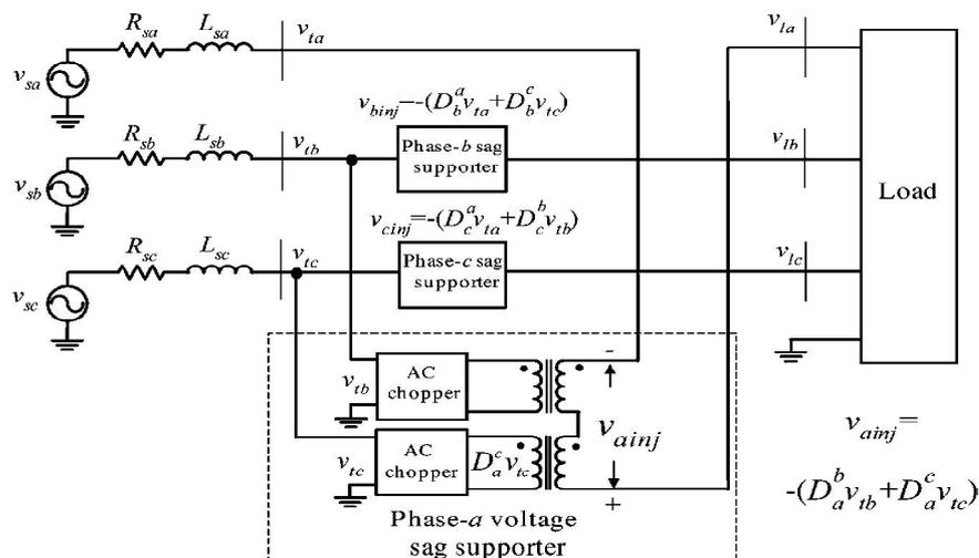
Fig. 5 Schematic diagram of the proposed inter-phase ac-ac voltage sag supporter
