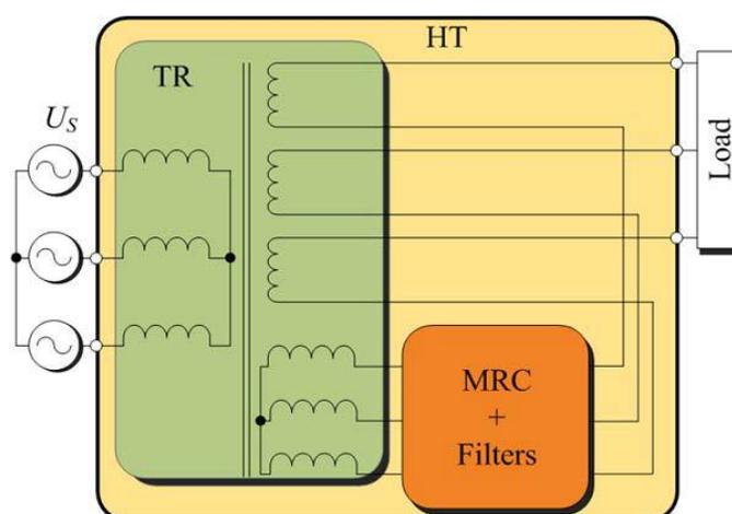
Fig. 6 Simplified scheme of three-phase HT
