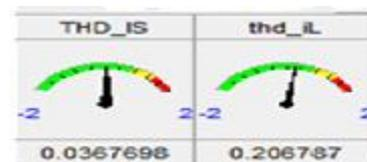
**Fig 4.4: THD of source and load current for existing method with PI Controller.**
