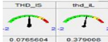
**Fig 4.1: THD of source and load current for conventional method without PI Controller.**
