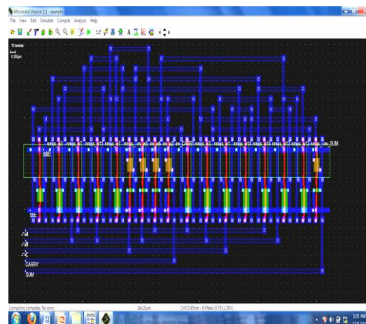
Fig9. Layout of CPL logic Full Adder
